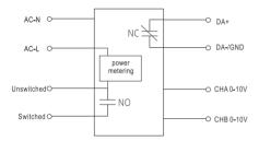
Note: The power output from Unswitched and Switched are both metering.
